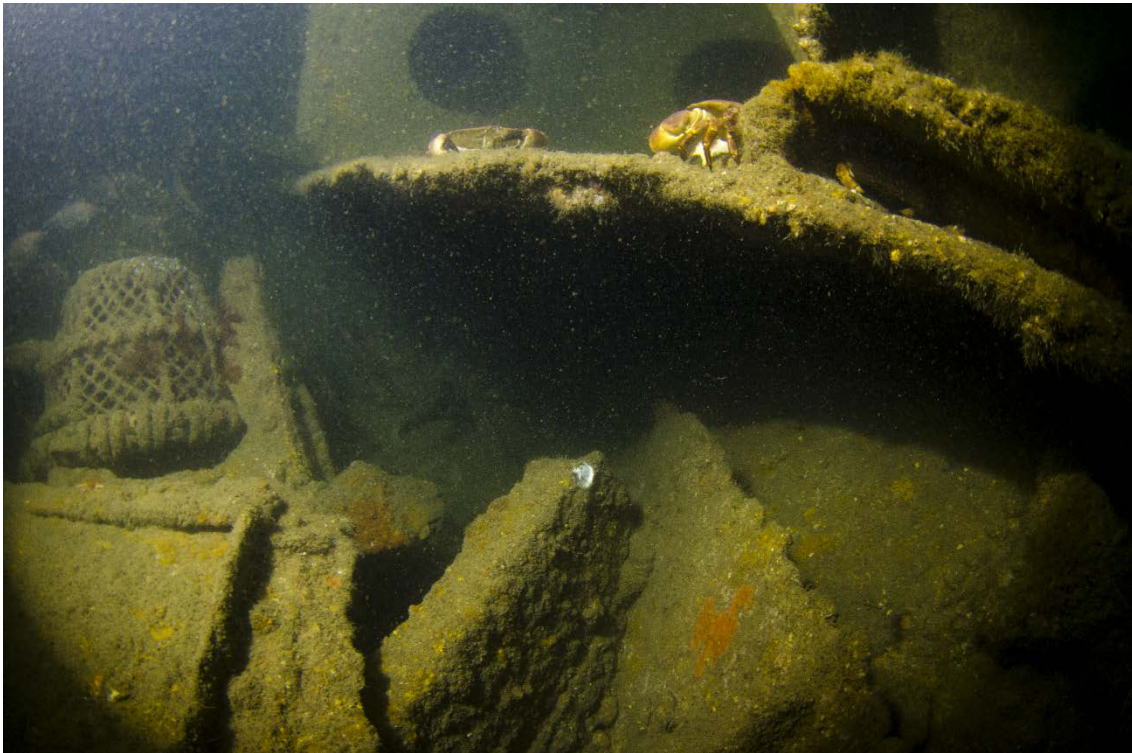
Figure 17: Circular plate that metal box of the gun reinforcement is riveted to
