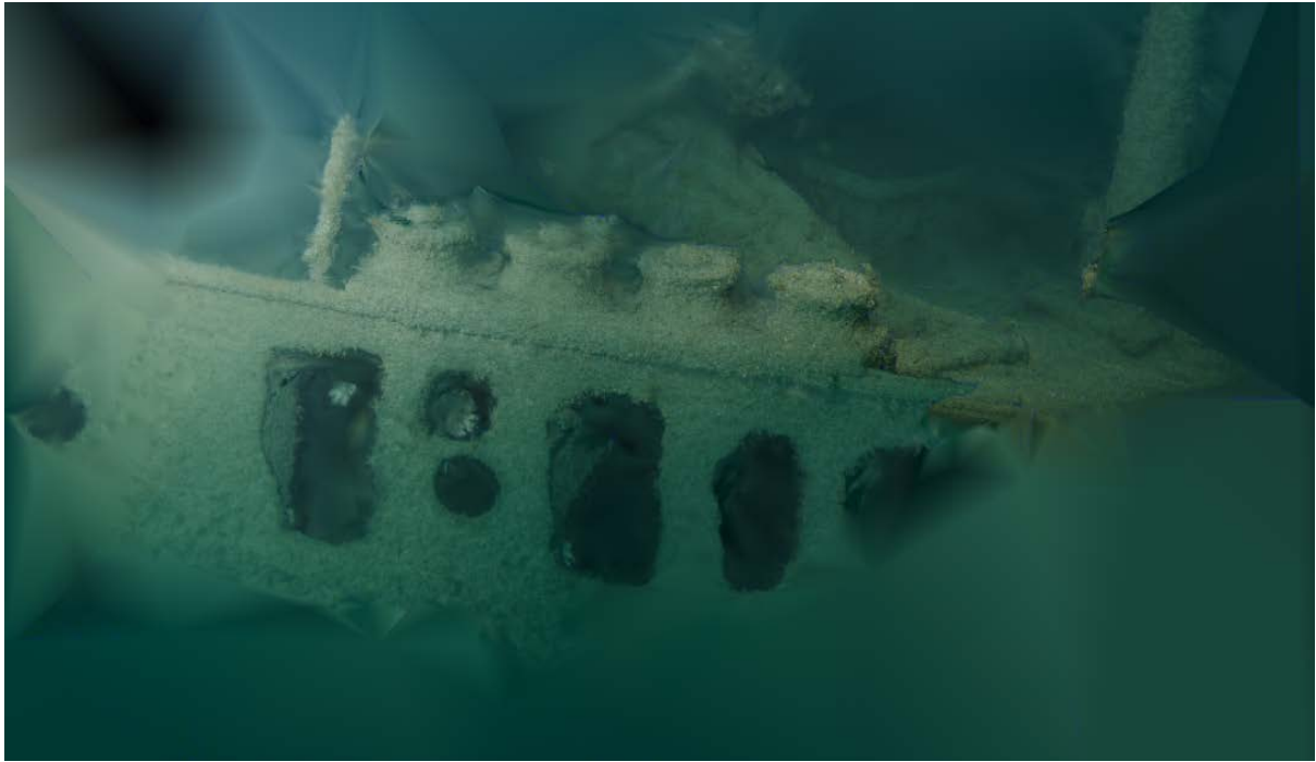
Figure 7: Row of mooring bollards at the bow (composite image modelled from a number of photographs).
