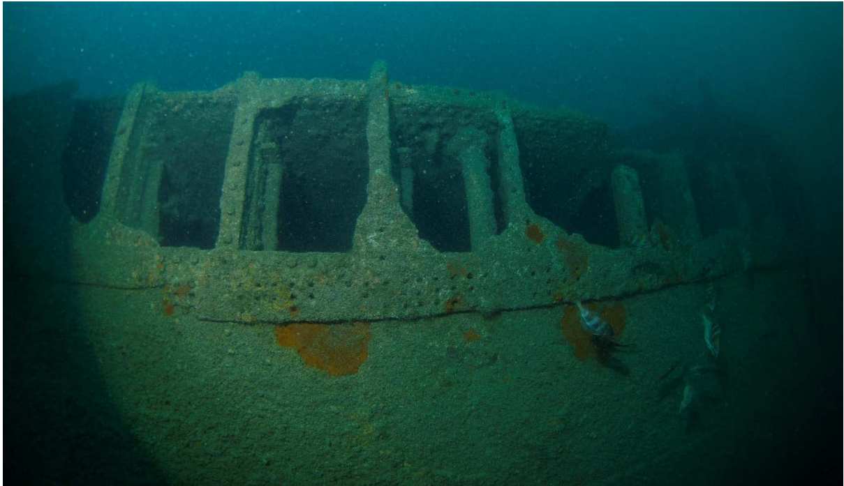
Figure 14: The hull framing and supports for upper deck structure.
